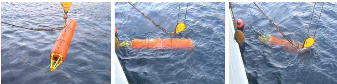
Figure 10. Cylindrical bottom mine launching from a surface ship
