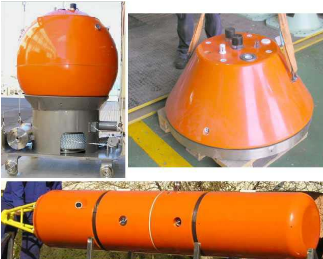
Figure 3. Advanced MINEA mine types: moored mine (upper left), low profile bottom mine (upper right) and cylindrical bottom mine (lower)
