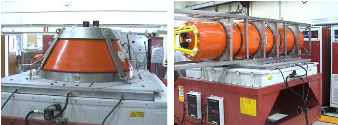
Figure 17. Vibration tests: Low Profile mine (left) and Cylindrical mine (right)
