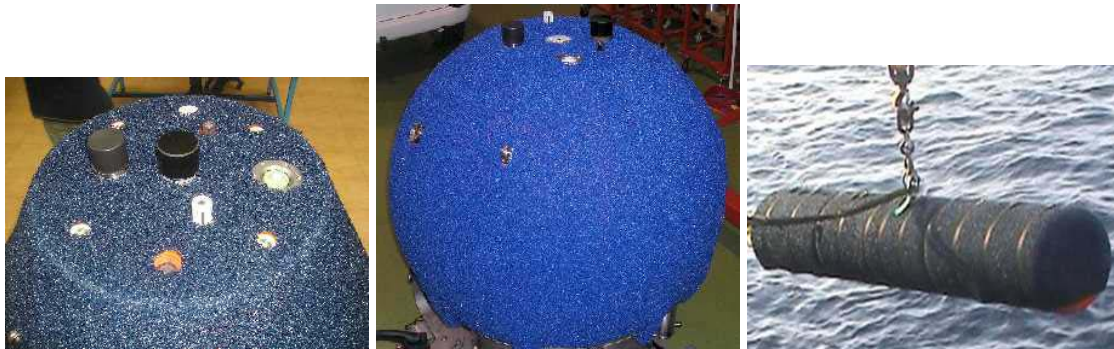
Figure 7. Anechoic coverings of the mines
