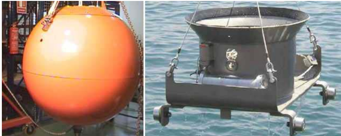
Figure 5. MINEA moored mine components: buoy (left) and sinker (right).
