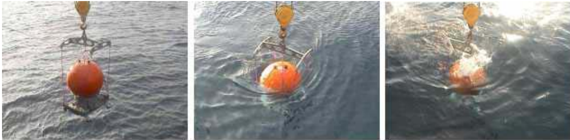
Figure 15. Moored mine launching from a surface ship using a specific launching tool
