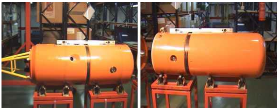
Figure 6. MINEA cylindrical bottom mine components: module 'A' (left) and module 'B' (right).
