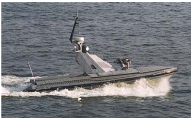
Figure 14. Unmanned surface vehicle (USV) PROTECTOR for the neutralization of underwater threats manufactured by Rafael
