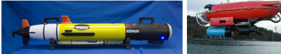
Figure 13. Unmanned autonomous vehicles. REMUS (UUV) manufactured by Hydroid (left) and PLUTO PLUS (ROV) manufactured by Gaymarine (right).
